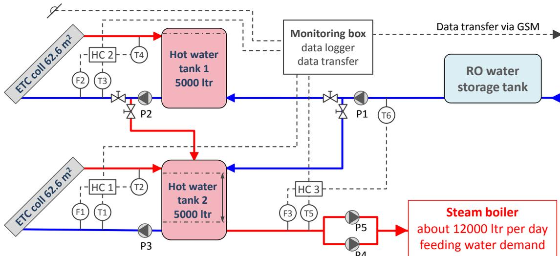
Figure 1 Scientific monitoring system to measure the yield of the solar water heating system and subsystems
