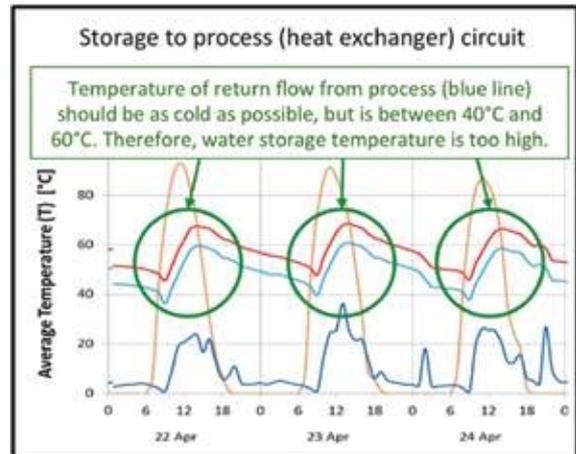
Figure 8 Temperatures of the storage to process circuit
