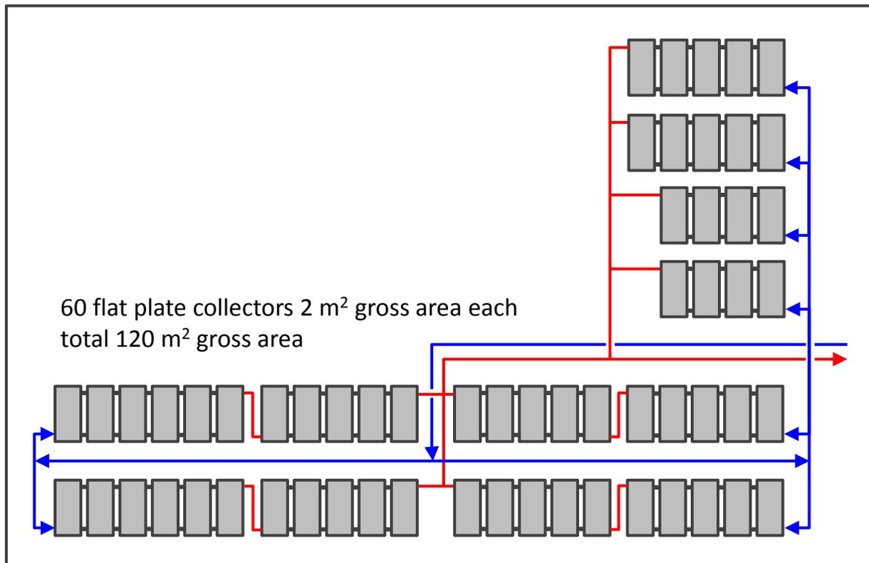
Figure 7 Hydraulic scheme of the collector field with 8 parallel connected collector rows
