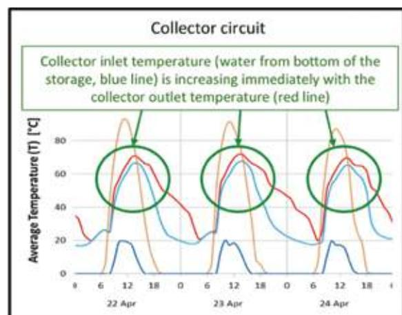
Figure 9 Collector inlet and outlet temperature curves
